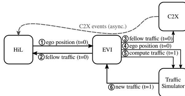
Figure 2. Architecture and data exchange of EVI and coupled simulators, from [4].
