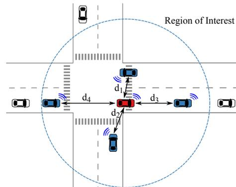
Figure 1. Dynamic floating ROI around the ego vehicle (in red, at the center). Communication is only simulated for vehicles within the ROI (in blue).
