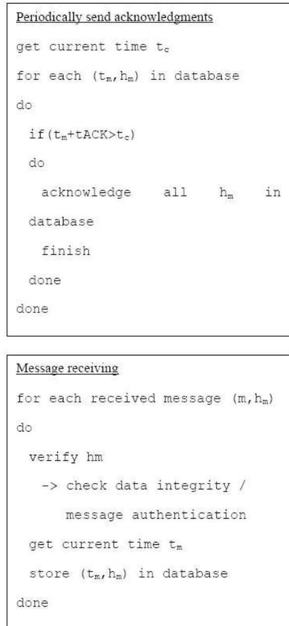
Figure 6: RAC implementation for the receiver
