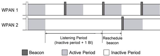
Figure 2. Illustration of beacon offsetting
