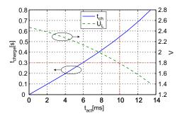
Figure 3. Dependency of the active period and the recharging time.
