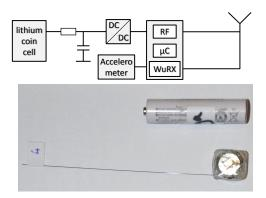
Figure 2. Hardware architecture and assembly of the mobile node.
