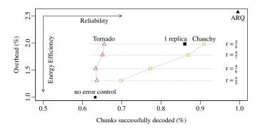
Figure 5. Reliability gain achieved by of the different error control strategies and code rates r versus their energy efficiency in terms of the necessary number of packet transmissions.
