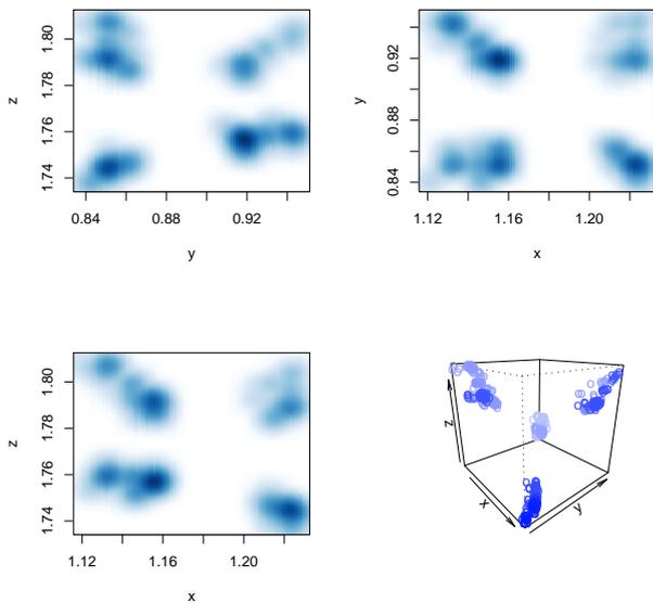
Figure 8. Localization accuracy: the quadrocopter is fixed in a position, the measured  $x, y, z$  coordinates are plotted
