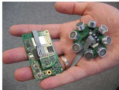
Figure 6. Ultrasonic measurement system with SunSpot node
