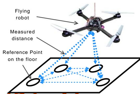
Figure 1. Four-rotor flying robot hovers over reference points
