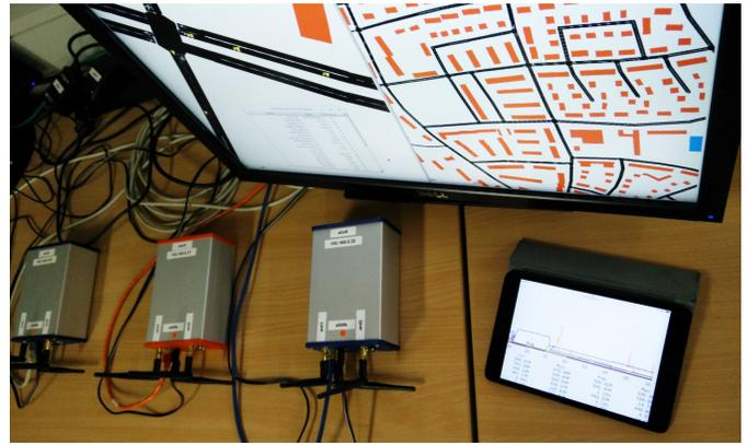
Figure 3. Photo of the experiment setup: the OBUs communicate via IEEE 802.11p among them. In the background, the position of the virtual prototypes in the road traffic simulation is visible. In the bottom right, an end user is logged into the WiFi access point of one of the OBUs, using a web browser to access a service offered via the network, on another OBU.
