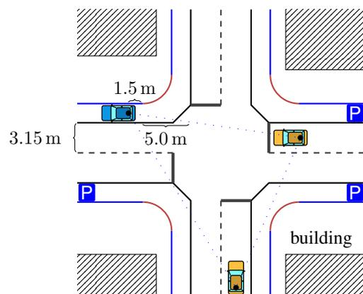
Fig. 1. Schematic view of the X intersection scenario.
