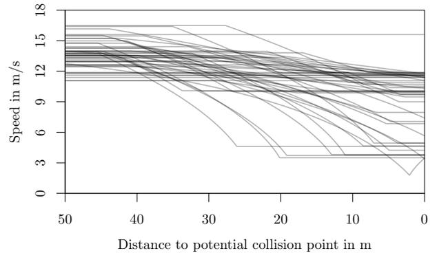
Figure 2: Vehicle dynamics of 24 exemplary intersection approaches of two vehicles.
