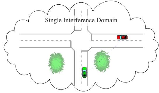
Fig. 3. Schematic overview of the considered scenario showing two approaching and communicating vehicles, that do not see each other yet. Vehicles causing network congestion are not shown.
