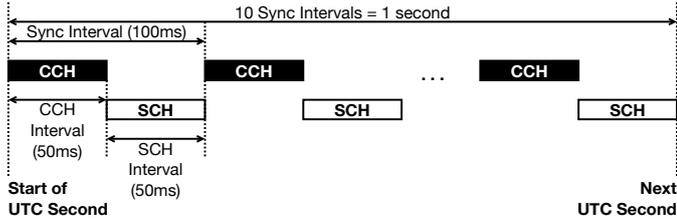
Figure 1: The principle of the WAVE Split Phase Protocol. A node periodically switches between the CCH and one of the available SCHs. Each node synchronizes its Sync-Intervals by GPS.
