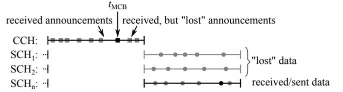
Figure 3: A node selects the best fitting SCH when an announcement is sent at  $t_{\text{MCB}}$ . Announcements received after this time are “lost” to the decision process. Similarly, data sent on other channels than the selected SCH is “lost” to the node.
