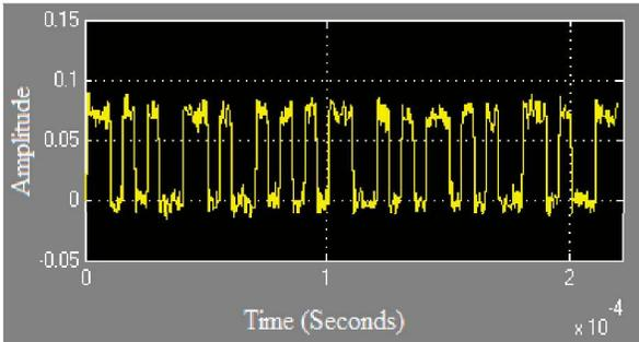
Fig. 4. Tag waveform with no collision
