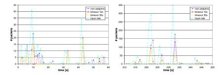
Fig. 10. Output rate for variable timeout and fixed detection ratio (10% whitelist, 1% blacklist)
