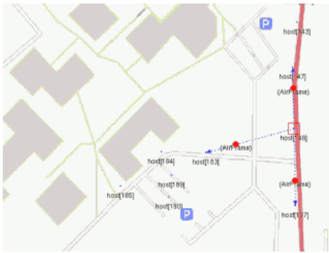
Fig. 5. Use of real-world data in bidirectionally coupled simulations. Model of a university campus running in the OMNeT++ network simulator and the SUMO road traffic simulator.
