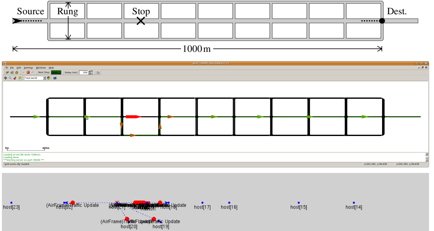
Figure 2. The simulated scenario and its graphical representations as rendered by the SUMO road traffic simulator and the OMNeT++/INET network simulator
