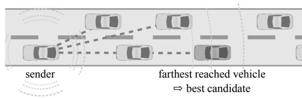
Figure 5. Conceptual idea of broadcast suppression using slotted 1-persistence.
