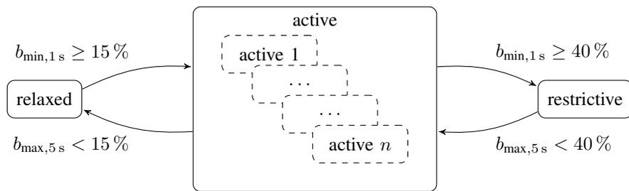
Figure 3. ETSI ITS G5 DCC state machine.
