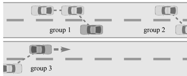
Figure 6. Principle of store-carry-forward between clusters of vehicles on a freeway.
