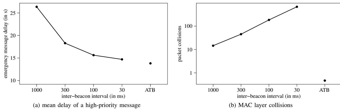
Figure 2. Beacons performance metrics recorded in the 16 km<sup>2</sup> grid scenario for various fixed beacon intervals as well as for ATB (for details of the simulation setup, please refer to [15]).
