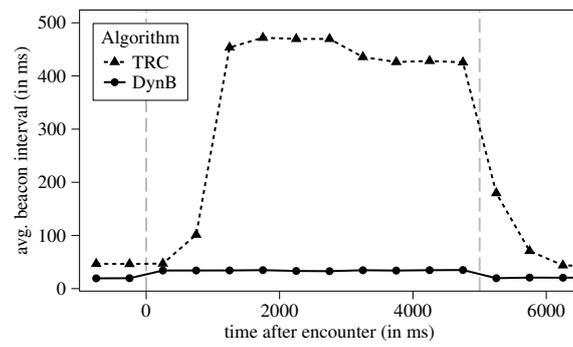
Figure 4. Comparison of the mean beacon intervals calculated by TRC and DynB when two initially disconnected clusters of vehicles meet (at time 0) and separate again (5000ms later). For details of the simulation setup, please refer to [31].
