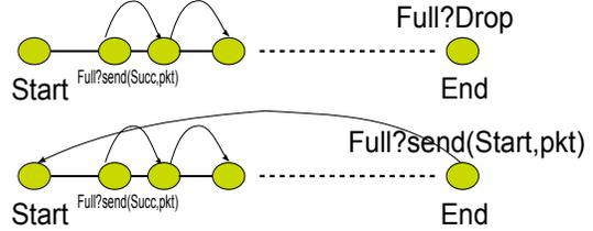
Fig. 3. VCP-based cooperative storage: Ring disabled (up) and Ring enabled (bottom)
