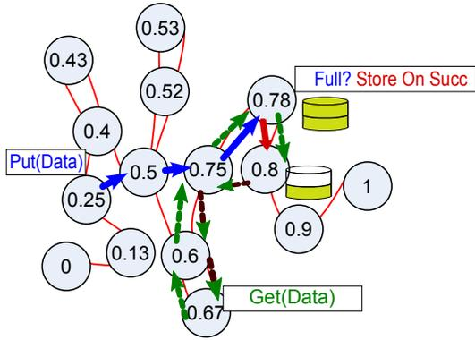
Fig. 4. An example for a inserting/retrieving data and using the successor on virtual cord to store data on behalf of a storage-exhausted node
