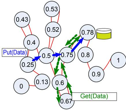
Fig. 2. An example for a Inserting/retrieving data using the virtual cord and greedy routing exploiting local neighborhood information
