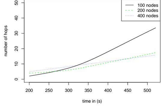
Fig. 9. Data insertion path length for different network sizes
