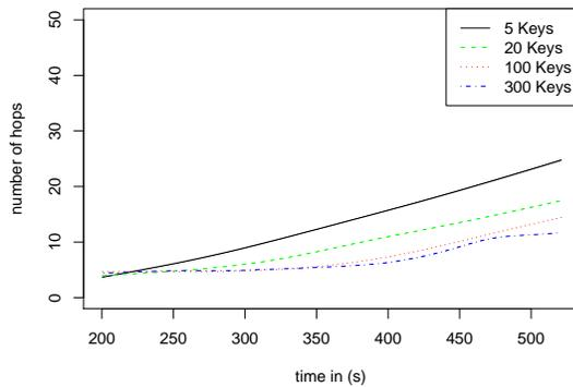
Fig. 10. Data insertion path length for different number of keys
