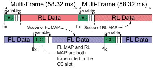
Fig. 2. L-DACS 1 resource allocation structure
