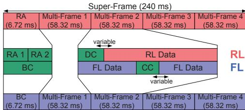
Fig. 1. L-DACS 1 frame structure
