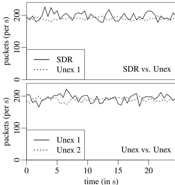
Figure 6: Throughput / fairness when saturating the channel with two devices (Unex and SDR).
