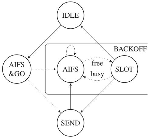
Figure 2: CSMA state machine implemented on the FPGA that controls frame transmission.
