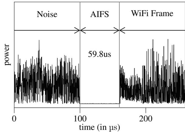
Figure 3: Power measurements to verify AIFS timing and to determine channel access delay.
