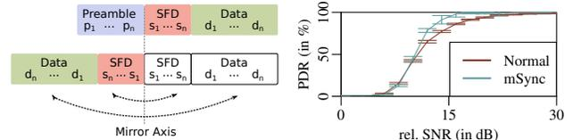
(a) Normal frame format (↑) (b) Packet delivery ratio in an office environment vs. mSync (↓).
