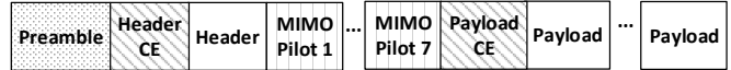
Fig. 2. PPDU structure of the PM-PHY with fields for frame detection, channel estimation and data transfer. The MIMO pilots and payload may consist of multiple blocks.
