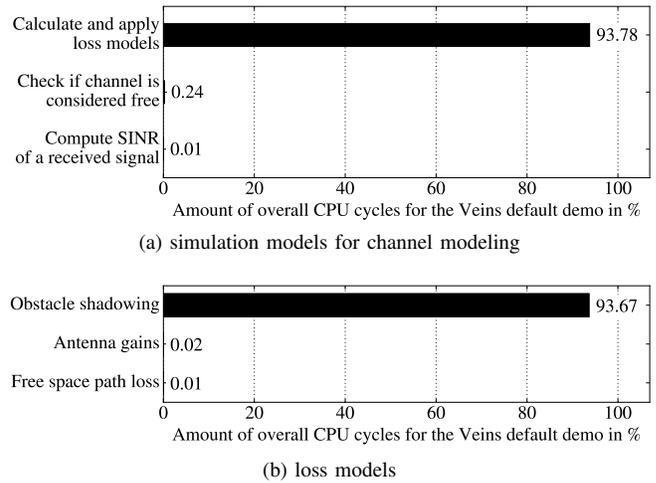
Figure 5. Results of profiling individual simulation components (by fraction of total CPU cycles).
