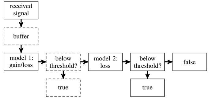
Figure 7. Steps performed in the proposed *thresholding* approach when receiving a signal: On-demand, iterative calculation of loss models to check reception power against a threshold – with short-circuit evaluation once a definite result can be determined. Steps added by the thresholding approach are highlighted.
