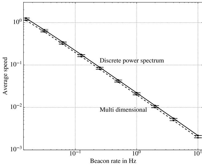
Figure 4. Average speed (computed simulation seconds per real time second) with confidence intervals (99 %) of the Paderborn scenario when using the multi-dimensional and discrete spectrum power model for signal representation in Veins for different beacon rates.
