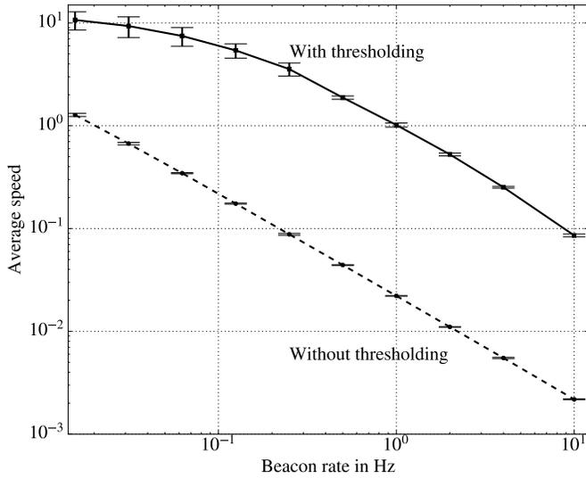
Figure 8. Average speed (computed simulation seconds per real time second) with confidence intervals (99%) of the Paderborn scenario when using the multi-dimensional and no thresholding and the discrete spectrum power model with thresholding in Veins for different beacon rates.
