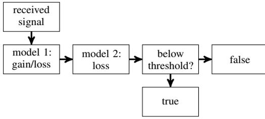
Figure 6. Common approach to checking whether the receive power level at a receiver exceeds a configured threshold in wireless network simulation: Application of all configured loss models to each received signal to derive its power level and checking the calculated power level against the configured threshold.
