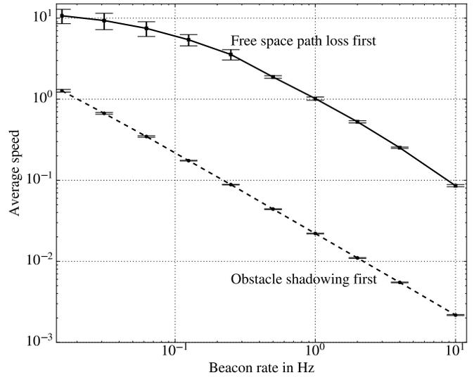
Figure 9. Average speed (computed simulation seconds per real time second) with confidence intervals (99%) of the Paderborn scenario with enabled thresholding mechanism for different beacon rates, but two possible orders of loss models.
