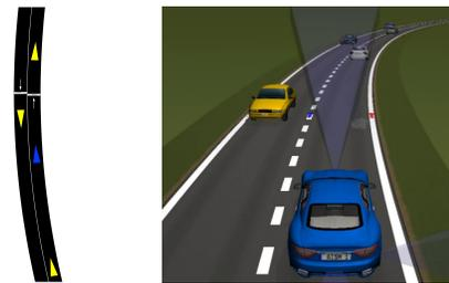
(a) Veins simulator (b) ASM real-time system
