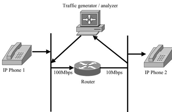
**Figure 8** Test environment for stress tests
