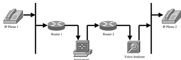
Figure 7 Test environment for QoS measurements
