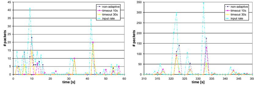
**Fig. 10.** Output rate for variable timeout and fixed detection ratio (10% whitelist, 1% blacklist)
