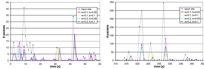
**Fig. 11.** Output rate for variable detection ratio and fixed timeout (10s)
