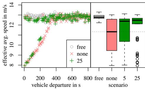
Fig. 2. Average speed of individual vehicles for free flowing traffic, traffic with an incident, and for broadcast-based IVC
