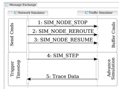
Fig. 1. Message exchange and time control between OMNeT++ and SUMO
