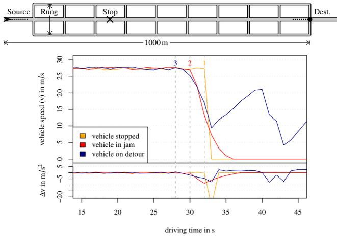
Fig. 6. Scenario description and speed / acceleration profile for vehicles approaching a congestion or taking a detour
