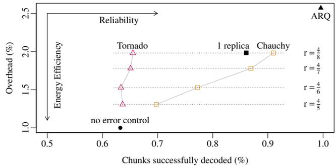
Figure 5. Reliability gain achieved by the different error control strategies and code rates  $r$  versus their energy efficiency in terms of the necessary number of packet transmissions.
