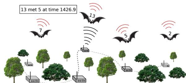
Figure 1. Conceptual scenario for bat tracking in the wild: stationary ground nodes are used to localize and to track bats based on emitted beacon messages. The mobile nodes are also used to monitor encounters and to download this data to the ground network to increase the observation range beyond the ground station area.
