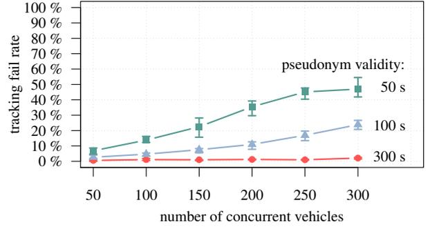
Figure 10: Chance of evading tracking in the blind-spot freeway scenario (beacon rate = 1Hz). Plotted are the averages over all simulation runs. Error bars extend from the 25% to the 75% quantiles.
