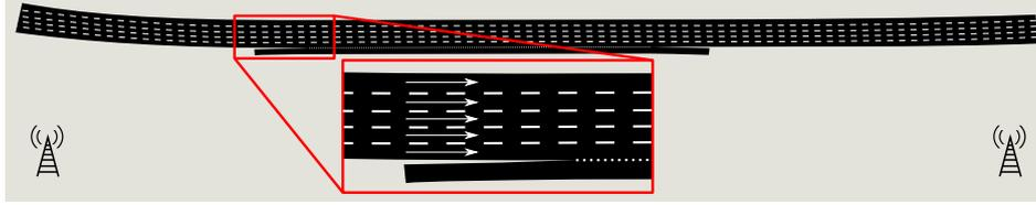
Figure 4: Highway 101 Scenario. Node movement is based on 900 s of real traffic on a 640 m stretch of Hollywood Fwy near Universal City Plaza, Los Angeles, CA. Five lanes are running in the same direction, temporarily joined by a sixth lane in the middle. Traffic was recorded by eight video cameras and post-processed to derive trace files [33]. An adversary is able to fully monitor the scenario.
