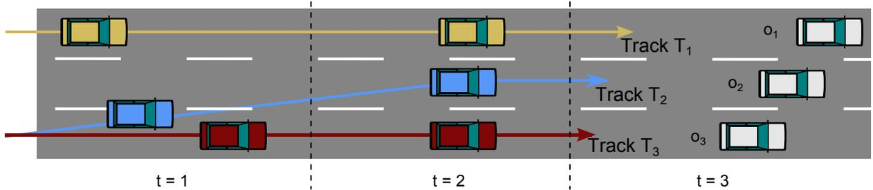
Figure 7: Tracking can be seen as the problem of assigning a new observation  $o_i$  to a track  $T_j$ .
