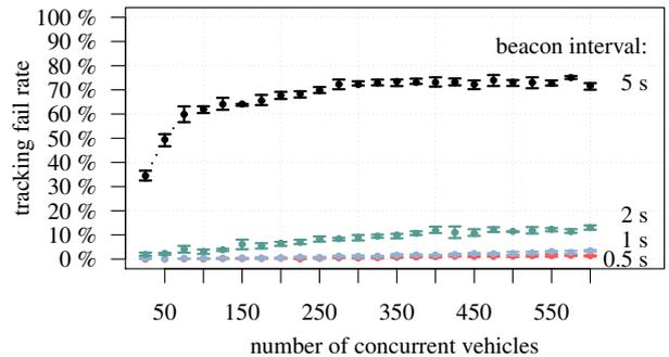
Figure 8: Chance of evading tracking in the synthetic grid scenario. Plotted are the averages over all simulation runs. Error bars extend from the 25 % to the 75 % quantiles.
