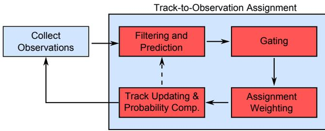
Figure 6: Architecture of a vehicle tracking system.
