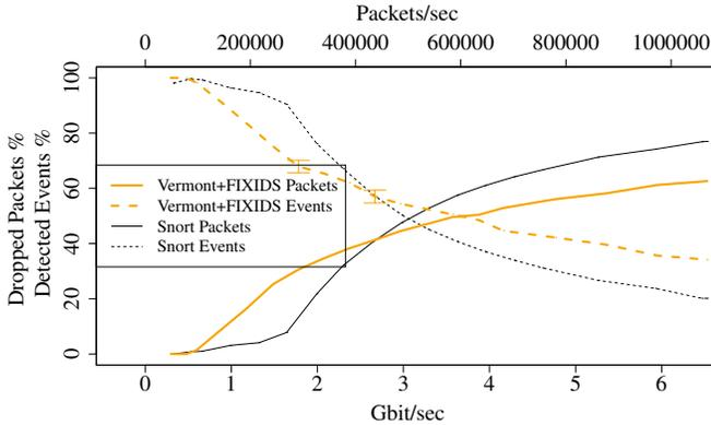
Fig. 3. Comparison of Snort and Vermont FIXIDS performing packet aggregation and intrusion detection on the same workstation receiving the proxy trace (plus 500 additional events)  $\times 5$  over the network at different packet rates. Average over 10 runs (confidence interval (95%) is shown if  $> \pm 2\%$ ).
