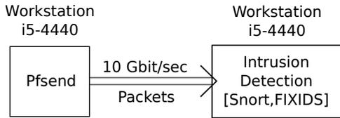
Fig. 2. Experiment setup with pfsend sending packets to Snort or FIXIDS doing intrusion detection. In this case FIXIDS also aggregates packets to IPFIX Flows before the intrusion analysis.
