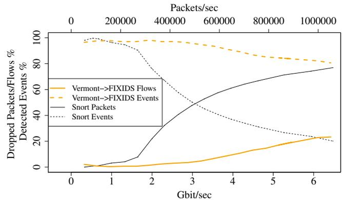
Fig. 5. FIXIDS receiving IPFIX Flows from a remote Vermont entity (over PR-SCTP) reading the proxy trace (plus 500 additional events)  $\times 5$  over the network. In comparison to Snort. Average over 10 runs (confidence interval (95%) is shown if  $> \pm 2\%$ ).
