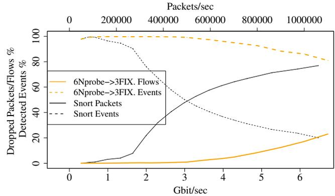
Fig. 9. 3 FIXIDS instances receiving IPFIX Flows from 6 remote Nprobe entities receiving the proxy trace (plus 500 additional events)  $\times 5$  over the network. In comparison to Snort. Average over 10 runs (confidence interval (95%) is shown if  $> \pm 2\%$ ).
