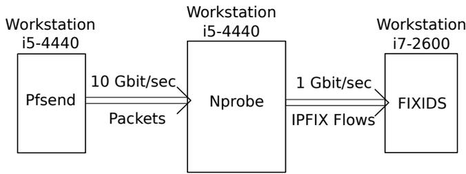
Fig. 6. Experiment setup with pfsend sending packets to Nprobe which aggregates the packets and sends Flows to FIXIDS.
