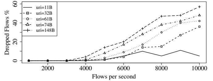
Fig. 10. Vermont FIXIDS performing intrusion detection on 100k IPFIX Flows with different HTTP Uri lengths at different Flow rates.
