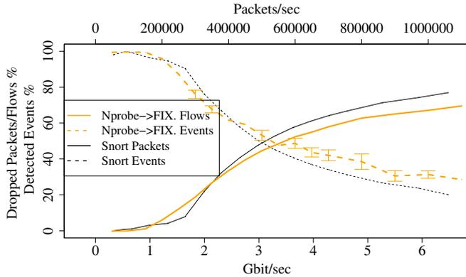
Fig. 7. FIXIDS receiving IPFIX Flows from Nprobe receiving the proxy trace (plus 500 additional events)  $\times 5$  over the network. In comparison to Snort. Average over 10 runs (confidence interval (95%) is shown if  $> \pm 2\%$ ).
