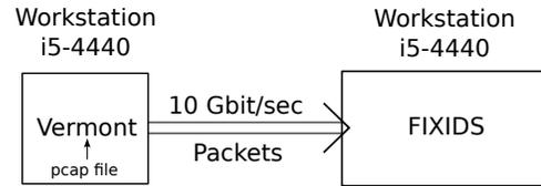
Fig. 4. Experiment setup with Vermont reading the prepared pcap trace file and sending the aggregated IPFIX Flows to FIXIDS.
