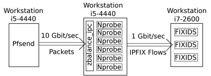
Fig. 8. Experiment setup with pfsend sending packets to 6 Nprobe instances which aggregate the packets and send Flows to 3 FIXIDS instances.
