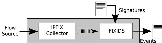
Fig. 1. Configuration of FIXIDS in Vermont
