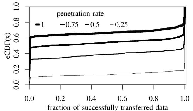
Figure 8: Success rate of transferring 1024 kB to a passing car during morning rush hour.
