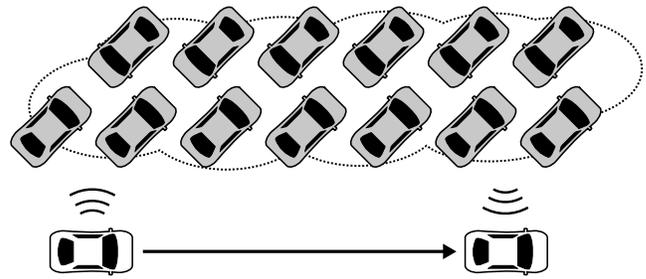
**Figure 1: A schematic overview of our approach where a driving car passes a cluster of parked cars forming virtual network infrastructure. The physical connection is automatically handed over among cars in the cluster as the driving car passes by.**
