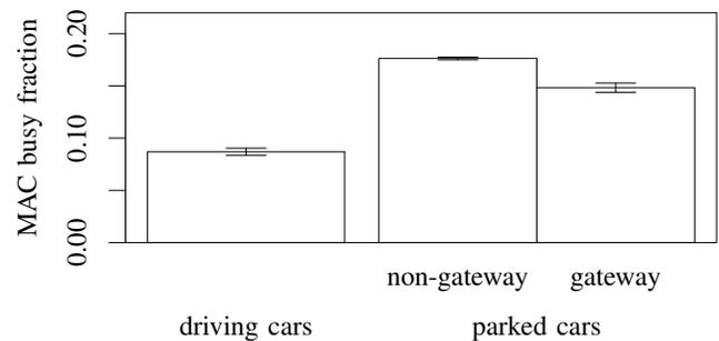
**Figure 4: MAC busy fraction including 95% confidence intervals for the single street scenario for the different types of cars.**
