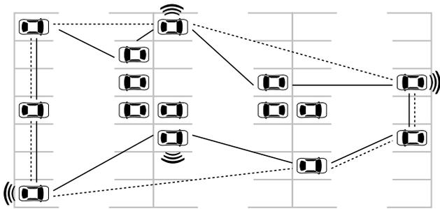
**Figure 2: Outline of the proposed algorithm for gateway selection.** First, the convex hull is computed (dashed line). Second, additional nodes are added based on the concave hull (solid line). Third, based on Algorithm 1, the gateway selection is performed.
