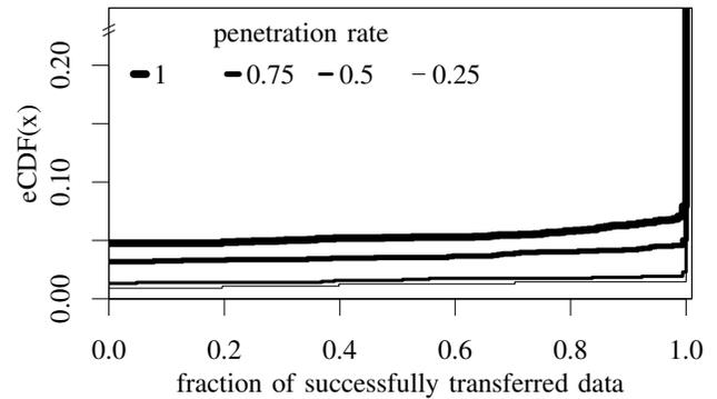
Figure 7: Success rate of transferring 128 kB to a passing car during morning rush hour in the realistic scenario.
