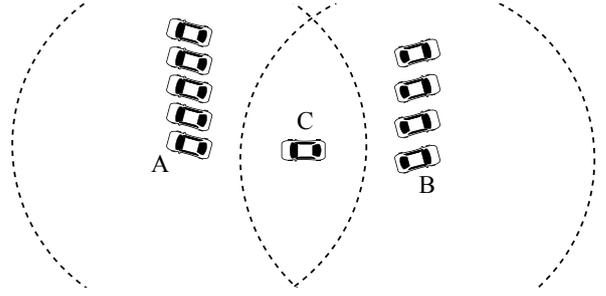
Figure 2: The stopping criteria for the gateway selection. If cars A and B are already a gateway and C is a candidate, C will not be added.
