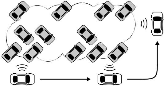
Figure 1: Schematic overview of our concept, where a driving car passes a cluster of parked cars forming virtual network infrastructure. The physical connection is handed over among gateways in the cluster as the driving car passes by.
