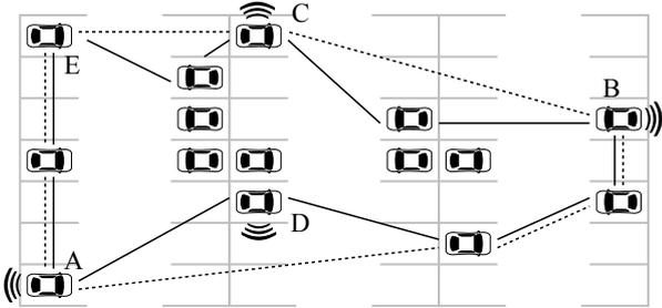
Figure 3: Outline of the proposed algorithm for gateway selection. First, the convex hull is computed (dashed line). Second, additional nodes are added based on the concave hull (solid line). Third, based on Algorithm 1, the gateway selection is performed.
