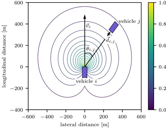
**Figure 2: Visual representation of our spatial model for calculating the weighting coefficient used for the AoI interpretation with an example configuration of  $\alpha = 0.75, \beta = 0.005$ .**
