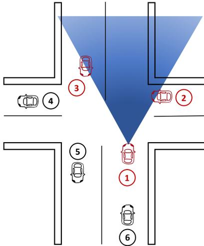
**Figure 1: Example scenario: Vehicles in the direction of movement of vehicle 1 (vehicles 2 and 3) are more relevant than others (vehicles 4, 5, and 6) when considering a safety application such as Intersection Collision Avoidance (ICA).**
