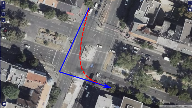
Figure 11. Intersection Mehringdamm/Gneisenaustraße: a traffic island obstructs the direct turn path (dashed line) and, thus, makes the indirect path (solid line) more likely to be used.
