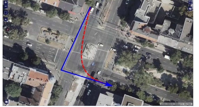
Figure 11. Intersection Mehringdamm/Gneisenaustraße: a traffic island obstructs the direct turn path (dashed line) and, thus, makes the indirect path (solid line) more likely to be used.
