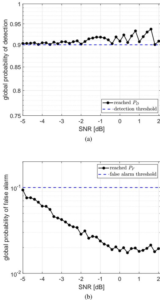
**FIGURE 5.** Detection constraints for different SNR. a) Global probability of detection. b) Global probability of false alarm.
