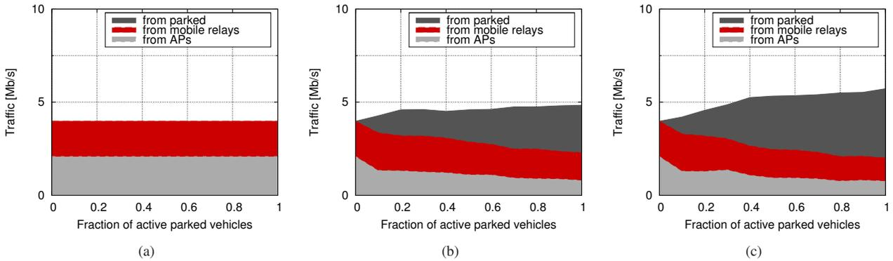
Figure 4. Traffic to downloaders for the cases “no park” (a), “no backbone” (b), and “with backbone” (c).
