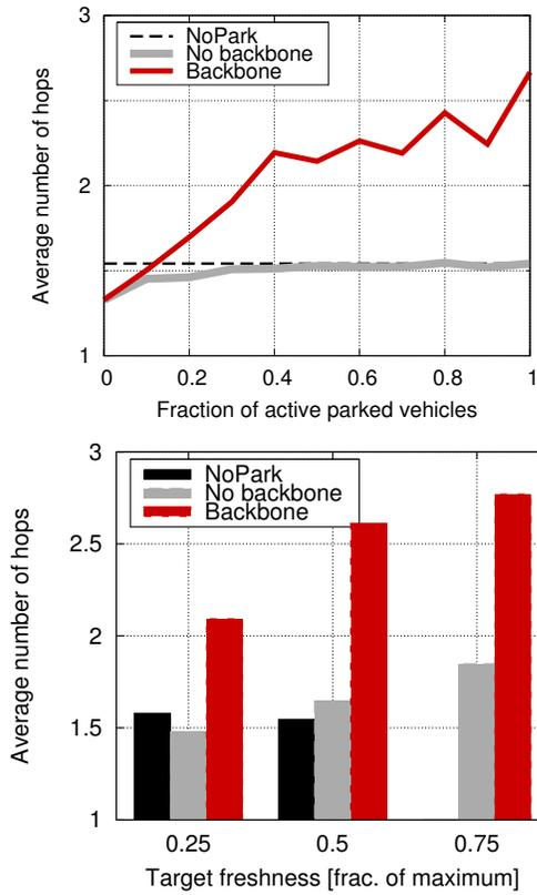
Figure 7. Average number of hops traversed by data traffic that downloaders successfully receive, when freshness (top) and idle time (bottom) are maximized.
