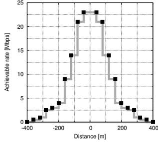
Figure 1. Characterization of the achievable network-layer rate as a function of distance, based on experimental data
