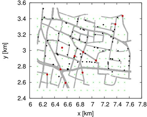
Figure 2. Road topology. Grey dots represent mobile vehicles, black dots represent parked vehicles, red ones represent RSUs. Green crosses mark the “check points”.
