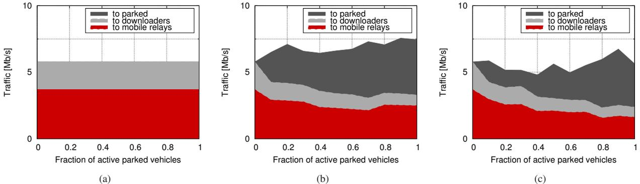
Figure 5. Traffic from RSU for the cases “no park” (a), “no backbone” (b), and “with backbone” (c).
