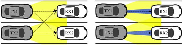
Figure 6: Simple scenario with four nodes: two transmitters (TX1 and TX2) and two receivers (RX1 and RX2); Yellow cones represent the whole radiation pattern; Blue cones represent sectors.
