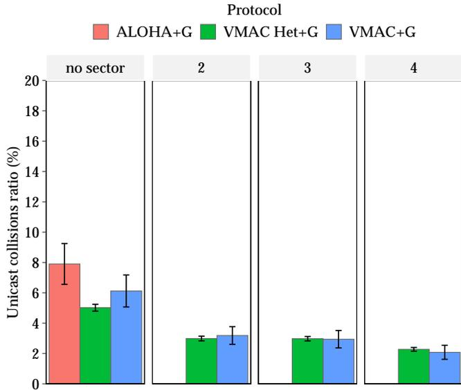
Figure 11: Ratio of colliding unicast messages for VMAC protocols with GPS feature. Different subplots show this metric for different number of sectors (noted above the corresponding plot). ALOHA does not support multiple sector configurations, hence only shown in the first plot.
