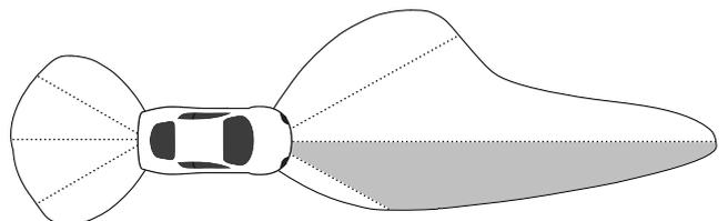
Figure 5: Illustration of the division of radiation patterns of lighting modules into multiple sectors.
