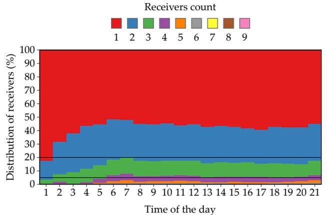
Figure 2: Distribution of the number of the receivers of a V-VLC message at different times of the day (i.e., Transmitter perspective).
