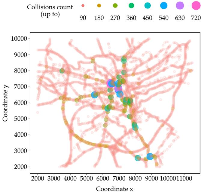
Figure 4: Two-dimensional density plot for the total number of collisions in the Luxembourg scenario. Size of the circle corresponds to the number of collisions.
