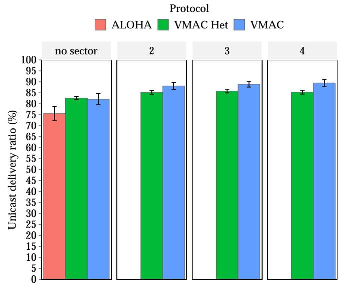
Figure 9: Delivery ratio for unicast messages for different protocols and varying number of sectors (noted above the corresponding plot). ALOHA does not support multiple sector configurations, hence not shown.
