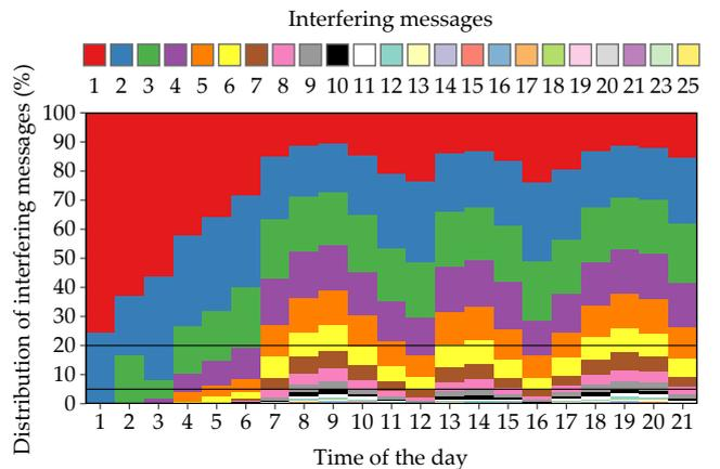
Figure 3: Distribution of the number of interfering frames for an ongoing V-VLC message reception (i.e., Receiver perspective).
