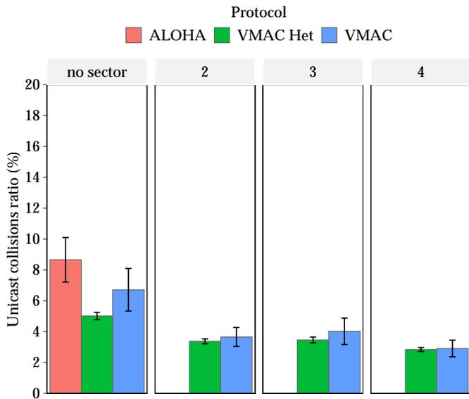
Figure 8: Ratio of colliding unicast messages. Different subplots show this metric for different number of sectors (noted above the corresponding plot). ALOHA does not support multiple sector configurations, hence only shown in the first plot.
