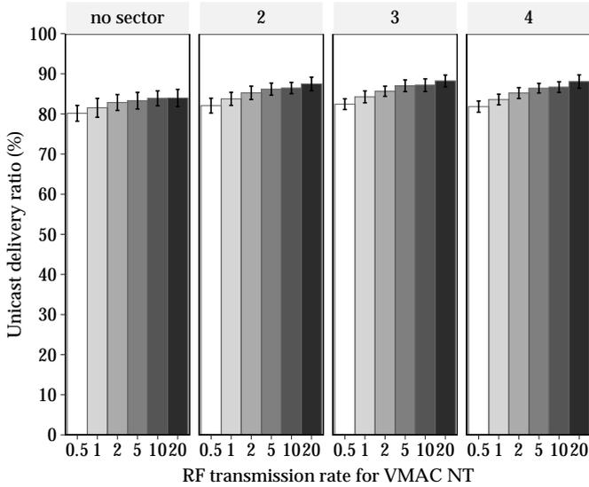
Figure 10: Unicast delivery ratio for V-VLC transmissions for the VMAC HET protocol for different RF transmission rate and number of sectors (noted above the corresponding plot).
