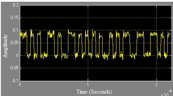
Fig.5. Tag waveform demodulated using respective carrier frequency (two tags collision)
