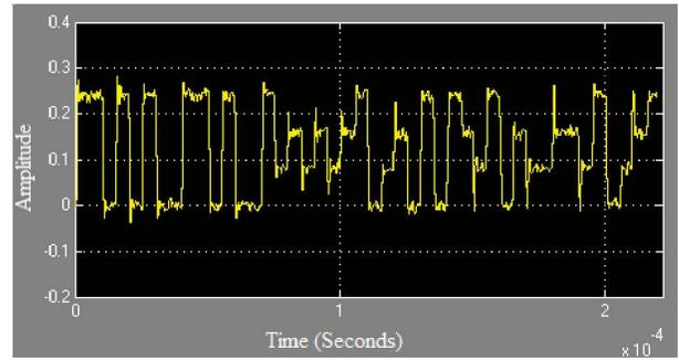
Fig. 6. Multiple tags using same carrier frequency (two tags collision)
