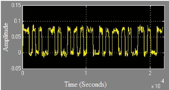
Fig. 4. Tag waveform with no collision
