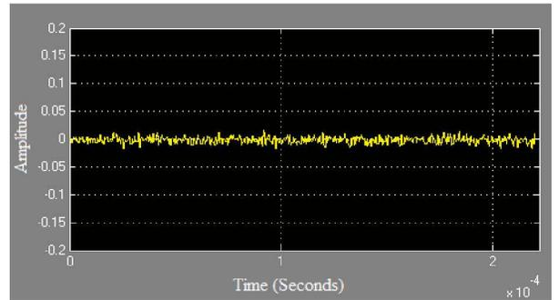
Fig. 7. Signal demodulated using carrier frequency not used by any of the tag
