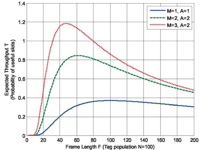
Fig. 2. Expected throughput  $T$  vs. collision recovery factor  $M$  for acknowledgments  $A \leq 2$
