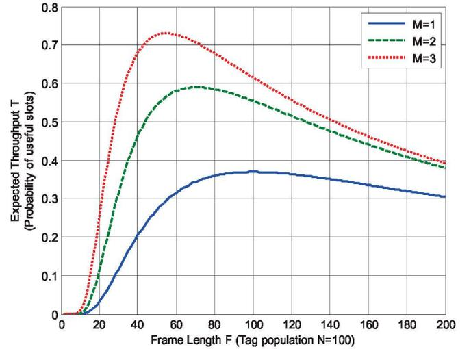
Fig. 1. Expected throughput  $T$  vs. collision recovery factor  $M$
