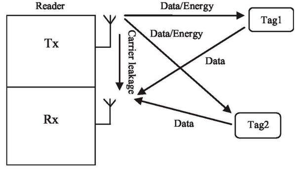
Fig. 3. Communication between an RFID reader and multiple tags
