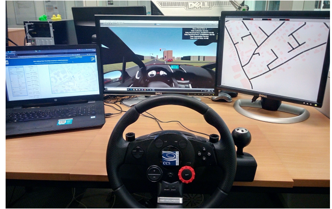
Figure 3. The laptop screen on the left shows Micro Cloud Web GUI which is connected to an Alix 3d3 system remotely. It shows a map, neighboring cars, and information about the micro cloud. On the central screen, a 3D driving simulator is running and the user can control the ego vehicle using a console. On the right screen, the SUMO simulation is running.
