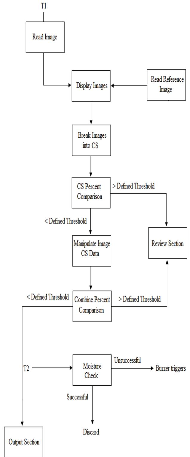
Fig. 2. Algorithm to handle the integration of digital image processing and moisturizing section
