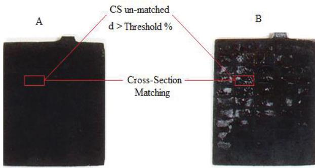
Fig. 3. Comparison of un-formed with standard reference plate image
