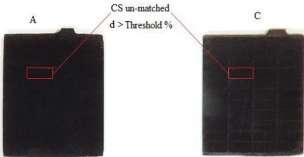
Fig. 4. Comparison of cracked with standard reference plate image
