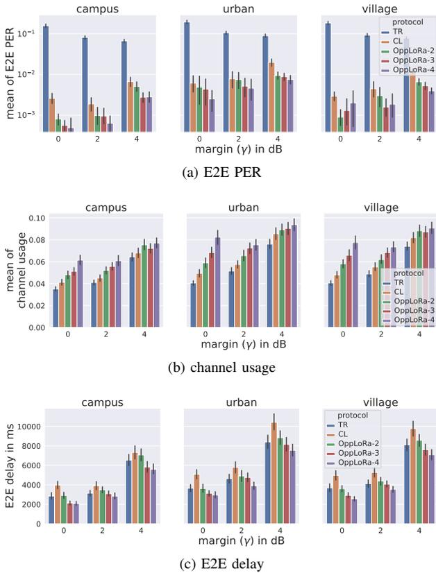
Fig. 4: E2E PER (logarithmic scale), channel usage and E2E delay for the three environments and node density 30 nodes/km<sup>2</sup>.
