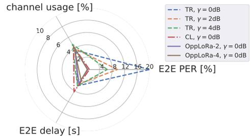
Fig. 6: Spider plot summarizing results for a node density 100 nodes/km<sup>2</sup> in urban scenario.
