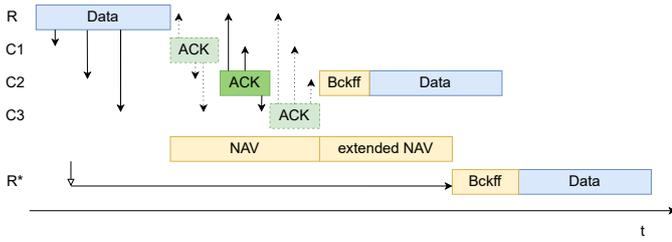
Fig. 3: Anycast-MAC in OppLoRa: slotted acknowledgments (ACKs) and virtual channel reservation using network allocation vector (NAV).
