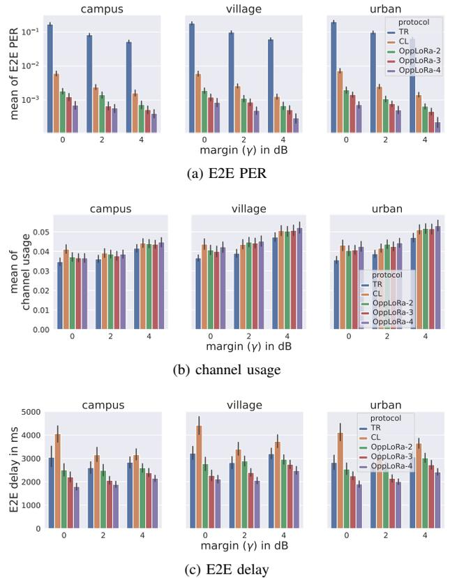
Fig. 5: E2E PER (logarithmic scale), channel usage and E2E delay for the three environments and node density 100 nodes/km<sup>2</sup>.
