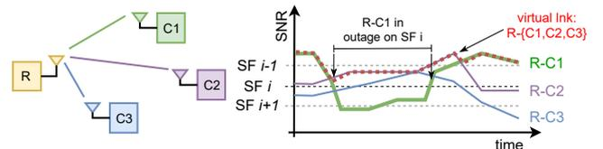
Fig. 1: Key idea: As the LoRa SF is fixed OppLoRa utilizes anycast transmissions to handle temporal drops in link SNR.
