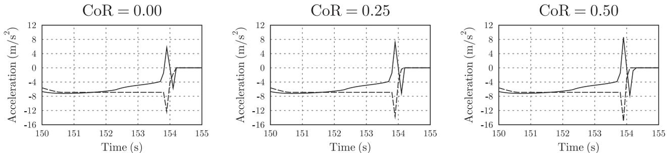
Fig. 9. Deceleration/acceleration profiles of a rear-end collision in the simulation, for different CoR values. The solid line represents the front vehicle, while the dashed line represents the follower.
