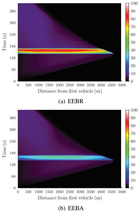
Fig. 7. Average loads as a function of the distance from the platoon head for 33 dBm transmission power, 5 lanes, reference speed 130 km/h.
