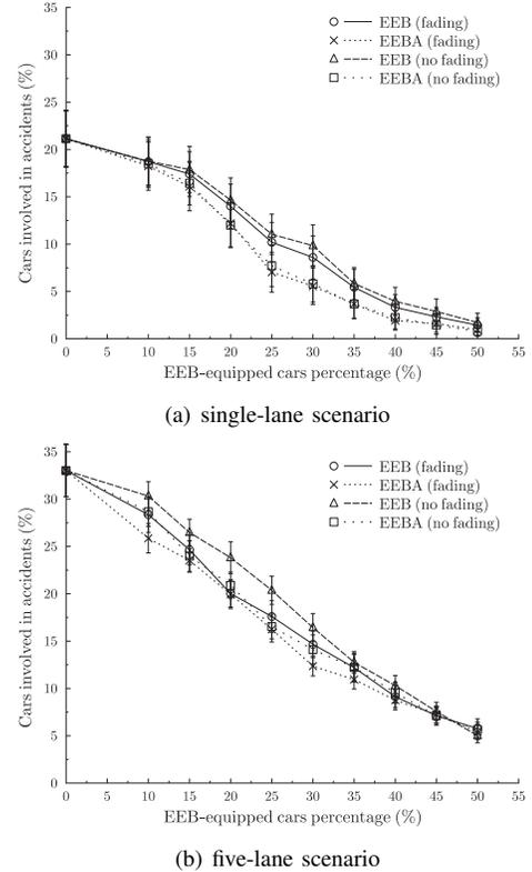
Fig. 8. Percentage of cars involved in accidents vs. MPR for the experiment with Nakagami fading, reference speed 130 km/h.
