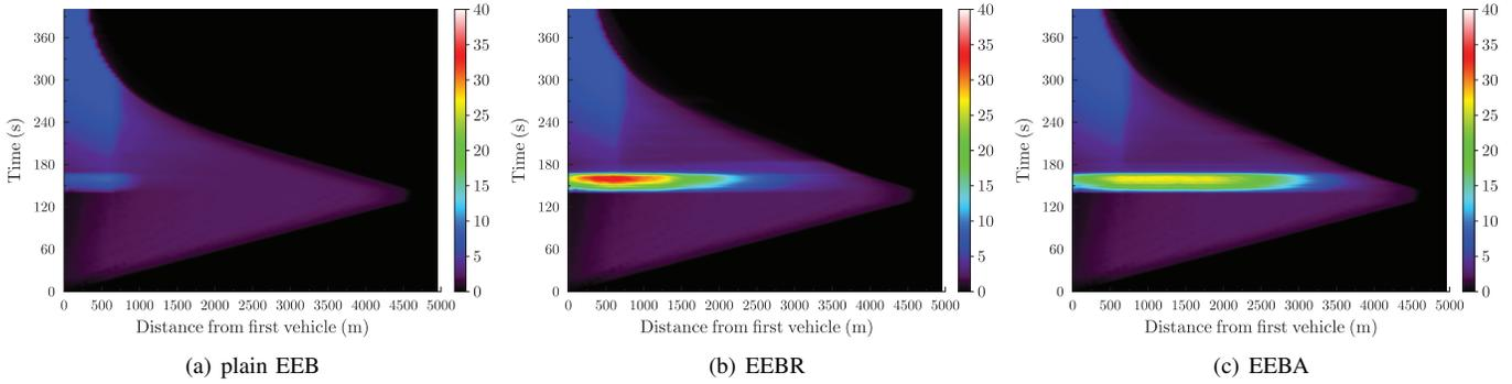
Fig. 2. Average load as a function of the time and the distance from the platoon head for the 5-lane scenario, average speed 130 km/h.
