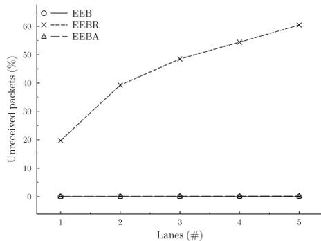
Fig. 1.  $l_{uf}$  as a function of the number of lanes for plain EEB, EEER and EEBA. The confidence intervals have been omitted for the sake of readability, since they were really small.
