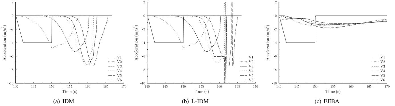
Fig. 5. Acceleration traces for three simulations, showing the first six vehicles in the first right lane, for 130 km/h reference speed and 5 lanes.
