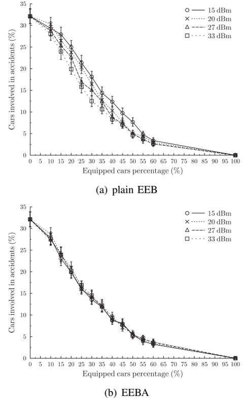
Fig. 6. Percentage of cars involved in accidents vs. MPR for different values of transmission power, 5-lane scenarios, average speed 130 km/h.
