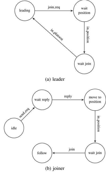
Figure 2. State machines of the sample join maneuver.
