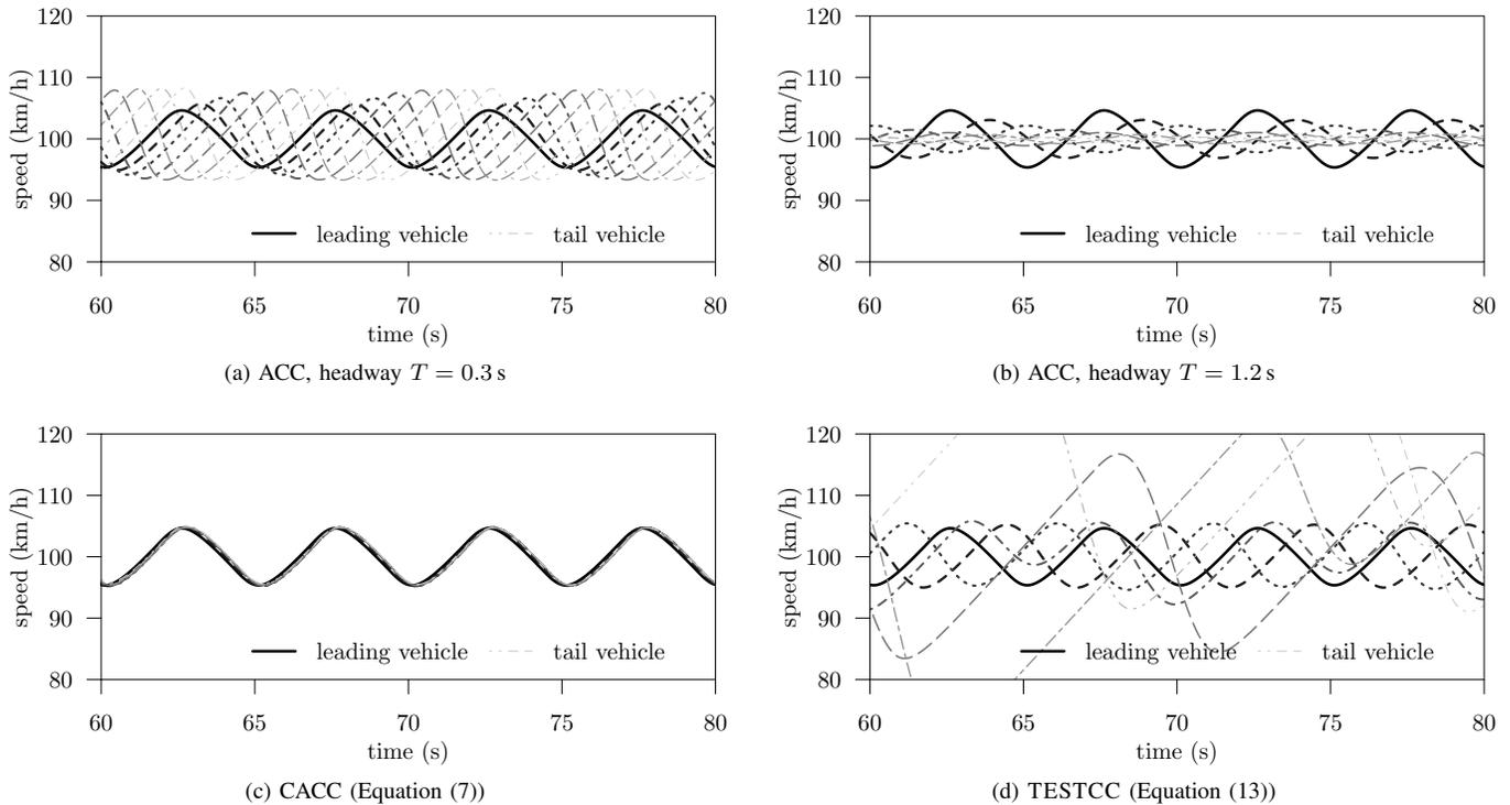
Figure 3. Vehicles speed for the different implemented cruise controllers showing string-stability properties.
