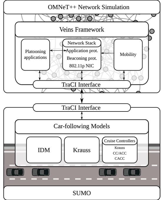
Figure 1. Schematic structure of the simulator.
