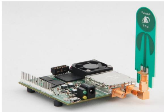
Figure 8.4.: P410 RCM with BroadSpec antenna (source: [40])
