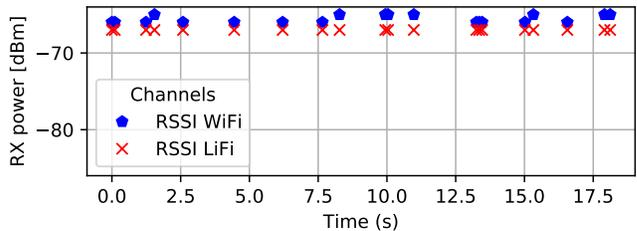
Figure 12. Hy-Fi under continuous RF signal jamming with deactivated interference management. Gaps indicate missing packets due to jamming.
