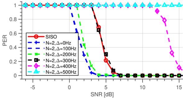
Figure 7. Impact of CFO on 802.11 transmission when two same signals with different CFO are received at receiver (MCS=0).
