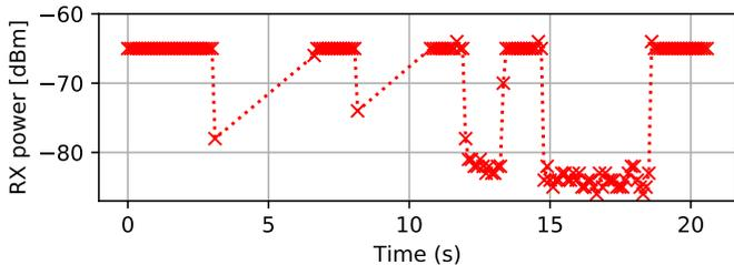
Figure 10. SISO-LiFi link with temporary signal blockage.
