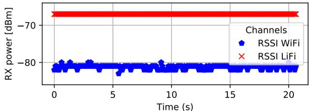
Figure 13. Hy-Fi under continuous RF signal jamming with activated interference management. No packet losses were observed.
