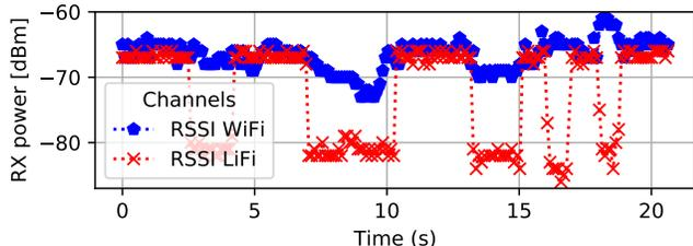
Figure 11. Hy-Fi link with temporary signal blockage.
