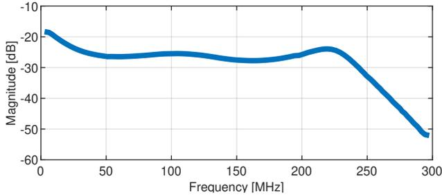
Figure 5. The magnitude response of the LiFi transmitter front-end
