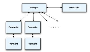
Figure 1.3.: Topology of the Vermont management system
